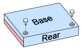
• Turn the router the right way up. Carefully pull the two halves of the router casing apart. The front panel may have a slight lip on it making it a little tricky – don't use brute force. Gentle wiggle the casing until it comes free.
