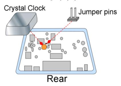
Placing the jumper with tweezers
